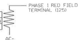
NOTE: The purpose of these resistors is to load the channel red monitor inputs in order for the Signal Sequence Monitor to use the full signal sequence monitoring capability on channels that do not use the red display in the field.
