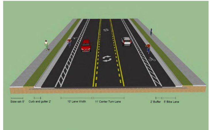
Typical Section with Turn Lanes
